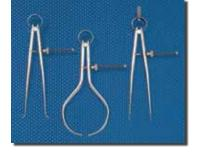
Designed for toolmakers and all good mechanics who require finer adjustment and better balance so a more sensitive feel can be obtained. The fulcrum stud is hardened and the bearing surfaces of the legs are large enough to prevent any side deflection. The bow spring is strong and flexible, and the adjustment is centrally located in the legs to assure smooth action.
