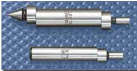
Work with flat, straight edges, shoulders, grooves, round work, studs, dowels, or center points and scribed lines can be accurately located with this handy tool. Double end model has a pointed contact at opposite end for locating center points and scribed lines. Body and contacts made of tool steel, hardened, ground and lapped to close tolerances for diameter and concentricity. Furnished in protective case.
