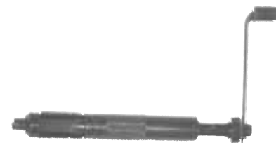
Type 2 - Hand Inserting Tool (Prewinder Tool)
