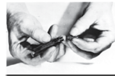
1. Slip screw into end of wrench.
