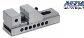
All surfaces hardened and precision ground to  $\pm$  .0002". Base and stationary jaw are one solid piece. Horizontal and Vertical "V" on moveable jaw for holding round work. Up to 400 lbs. pressure at 45° downward angle keeps work rigid. Quick adjustment is made by pulling pin and pushing sliding jaw forward -then tightening with an Allen wrench.
